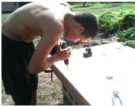
Figure 1. A Land Grant intern drilling holes in the polystyrene for the net pots. Figure 2. Apela's grandson drilling screws into the tray bottom to secure the 2x4's to it, making a box.
