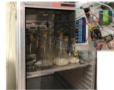
Figure 3. A commercial proofer is retrofitted with sensors and controllers (image insert) to produce fermented BSFL meals in an array of flasks for fish trials.
