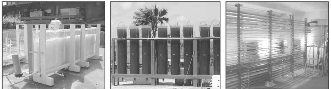
Figure 1. Large-scale photobioreactor systems, including (left) a 500-L flat-panel bioreactor at OI, (center) an OI cylinder-based air-lift bioreactor design, and (right) a tubular photobioreactor system.
