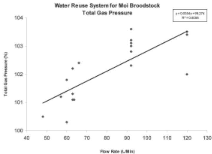
FIGURE 5. Total gas pressure (% saturation) of water from a moi broodstock tank with water flow ranging from 45–120 L/min.
