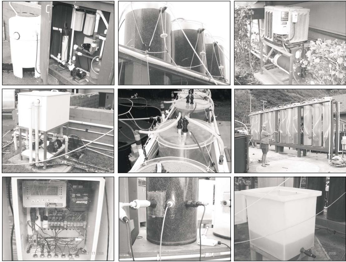
**FIGURE 2.** Photographs of the OI prototype columnar air-lift bioreactor system showing (a) the water purification and dosing system, (b) in-line air filters and algal harvest lines, (c) chiller unit, (d) chilled water circulation pump and reservoir, (e) cold-finger inflow and outflow lines, (f) chiller fingers in empty cylinders, (g) water quality monitor and control unit, (h) pH, temperature and dissolved oxygen probes, and (i) algal harvest container.
