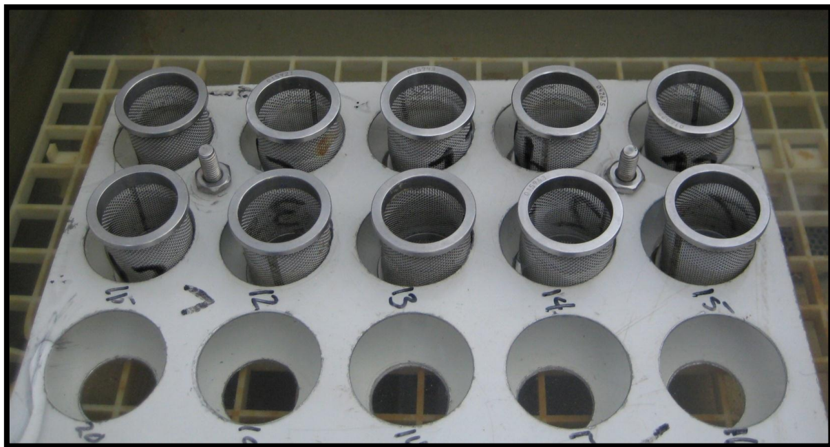
Baskets (without stoppers) & Rack set in water bath
