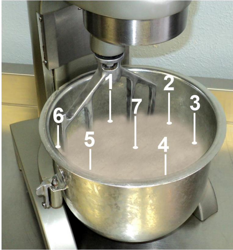
Sampling pattern for the Hobart Mixer (7 locations)
