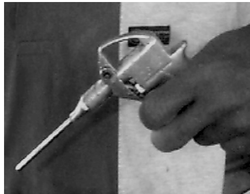
Figure 46. Oxygen nozzle used for inflating shipping bags. (Larry Sharron)
