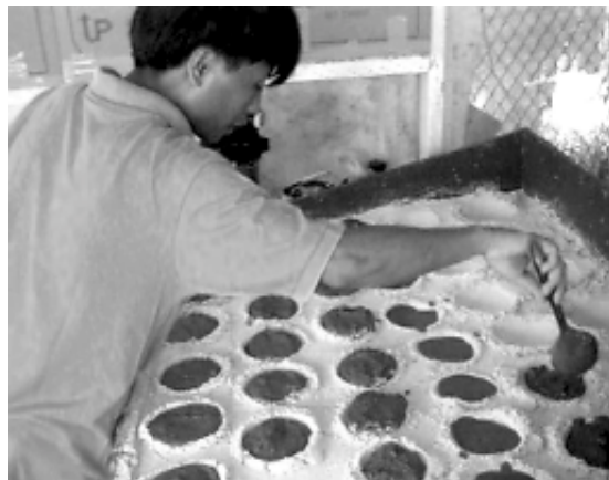
Figure 25. Pouring concrete recruitment substrates. (Simon Ellis)
